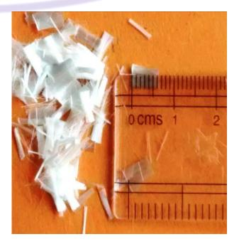
Note: The addition of fibers to a given mix may appear to decrease the slump. The workability, however, will not be affected and additional water should not be added.
